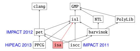
isl: manipulates parametric affine sets and relations barvinok: counts elements in parametric affine sets and relations pet: extracts polyhedral model from clang AST isa: prototype tool set including
